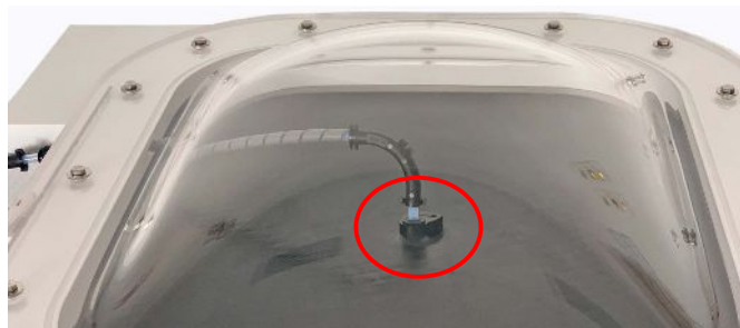
Fig. 6: Ratchet clamp on the top of the measuring chamber
