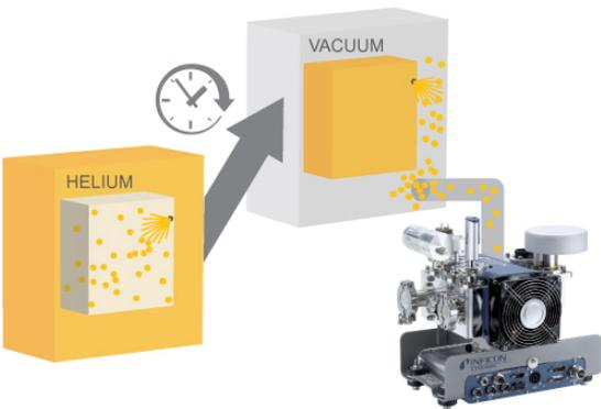
Battery cells that cannot be prefilled with helium are typically tested via bombing followed by vacuum chamber leak detection. This process is mainly used for prismatic and pouchtype cells.
