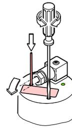
While depressing the pin with the cylindrical pin, adjust the <HV> potentiometer ...
