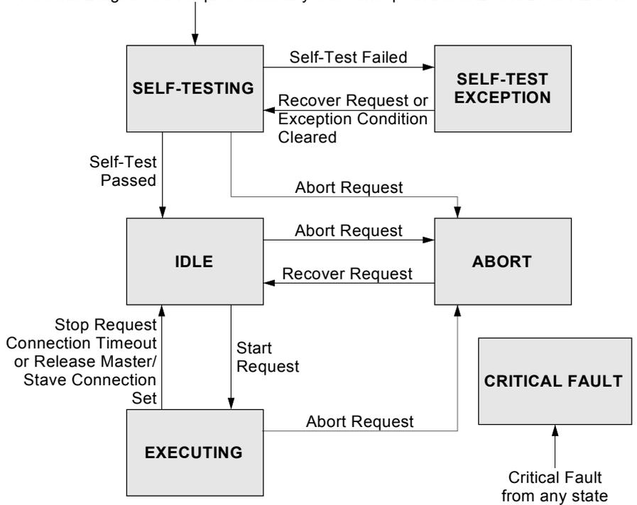
**Abort** - Used to transition the device application objects to the aborted state. This service request may be (and generally will) originated internally, from application objects.
