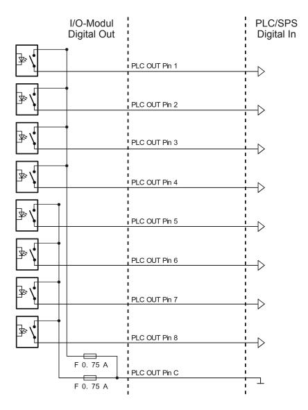
Fig. 3: Sample wiring, digital outputs
