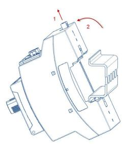
Fig. 7: Removing the I/O module
