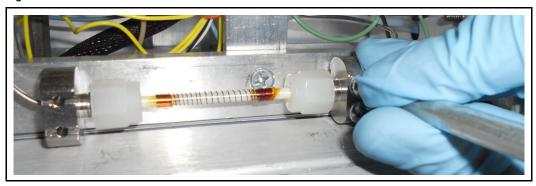
11 Ensure that the concentrator is fully seated into the left concentrator elbow. Using a 7/16" wrench, tighten both nuts by 1/4 of a turn. See Figure 13.
