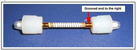
9 First, ensure the concentrator ferrules are properly oriented. Place the ungrooved end of the concentrator in the left concentrator elbow. Then, place the grooved end of the concentrator into the right concentrator elbow. Gently push the right elbow toward the left to seat the concentrator. While maintaining pressure on the right elbow, tighten both the left and right nuts until just finger tight. See Figure 11.
