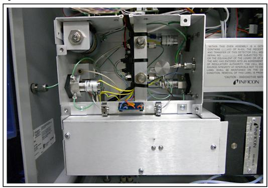
**5** Hold the sides of the concentrator board as shown. Gently remove the concentrator board by pulling outwards. See Figure 5.
