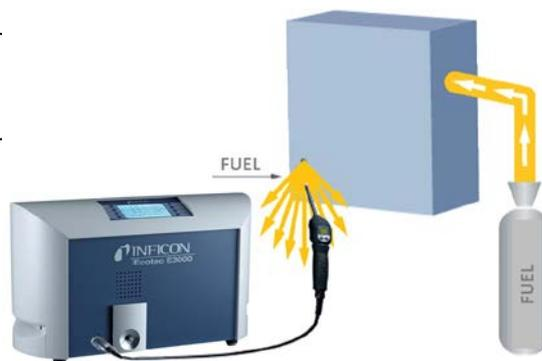
After final assembly of the fuel rail system, the connectors from the fuel rail subassembly to other components (like the high pressure fuel pump or the sealing of the fuel injector / fuel rail assembly against the engine block) need to be tested.
