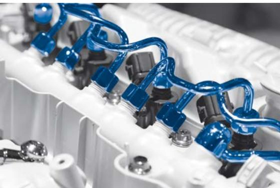
The need for lower fuel consumption drives the need for high pressure fuel injection. Injection pressures have significantly increased over the past few years. Today injection pressures can reach up to 2,000 bar (~ 150,000 psi). Fuel leaks can negatively influence fuel consumption and could cause a fire in the engine compartment. With increasing fuel injection pressures, larger leak rates will be generated by the same size leak hole.
